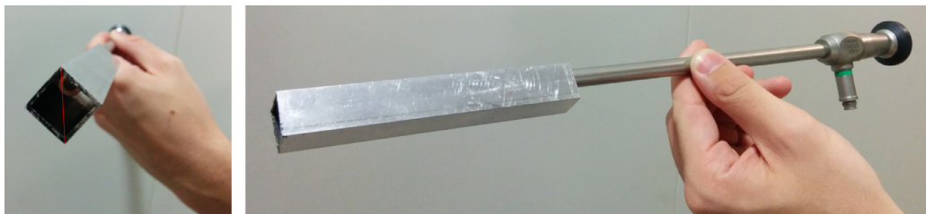
Fig. 10. A square-profiled tube rests on the distal part of the endoscope. The line passing by the top and bottom corners (red) intersects the sought axis of revolution. (For interpretation of the references to color in this figure legend, the reader is referred to the web version of this article).
